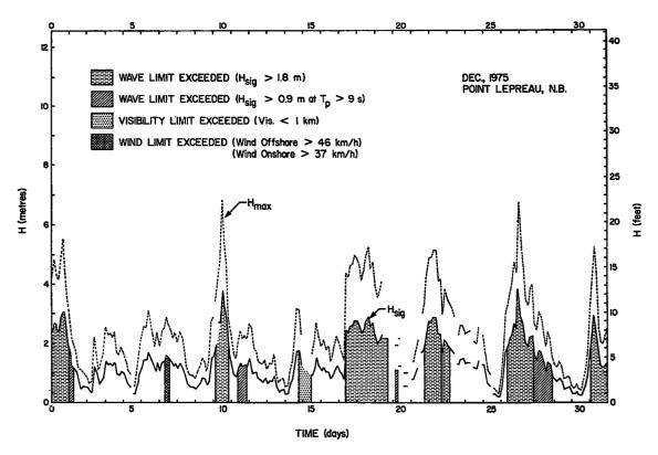
Figure 7. December 1975 wave record at Point Lepreau showing periods of down time.
