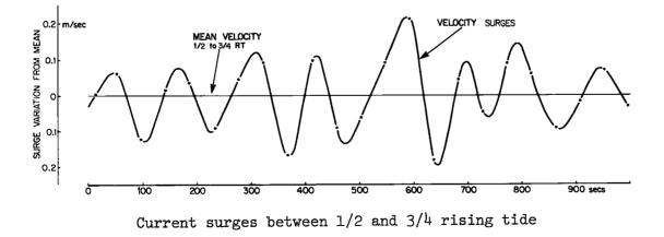
Figure 9. Current data taken 2 km off Tiner Pt., 27 August 1958.
